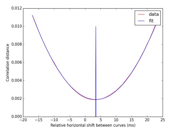
The red curve is the actual data, and the blue curve is a polynomial fit to the red curve, with the actual minima determined from the fit curve to increase precision.
