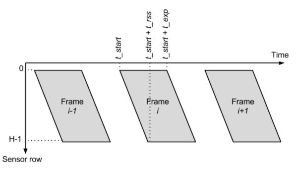
The first step in computing the camera rotation samples is to assign a single time to each frame. This is computed as the "middle" time for that frame, which in the above figure corresponds to a point in the exact center of each parallelogram. The equation for this is:
